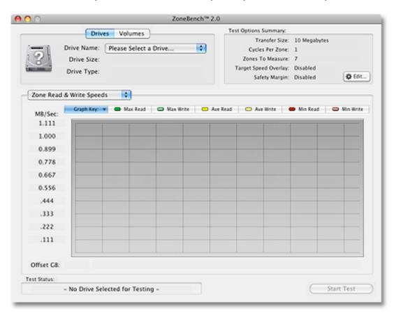
ZoneBench was created with maximum flexibility in mind. All zone test variables can be easily modified to suit almost any testing situation. Test results can be saved into tab-delimited text files suitable for importing into your favorite spreadsheet application or word processor.
