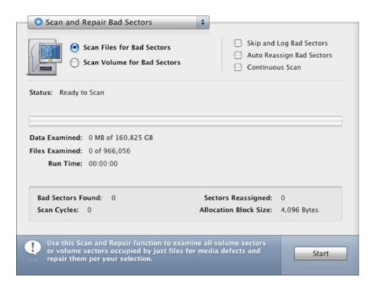
There are two alternative methods to detect defective sectors: scanning the files on a volume (Scan Files for Bad Sectors), or scanning the raw sectors on a volume (Scan Volume for Bad Sectors). Both methods have distinct advantages and some drawbacks which we will detail later in this section.
