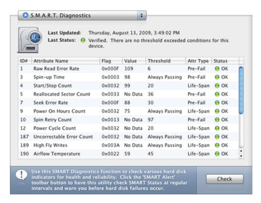
**NOTE:** Not all disk devices and/or interfaces support S.M.A.R.T. diagnostics. Currently, the Macintosh and its drivers support S.M.A.R.T. on ATA and SATA devices exclusively. S.M.A.R.T. capability on FireWire and USB interfaces is **NOT** supported.
