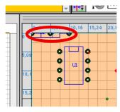
In the scheme, click on a component. Notice that it becomes red in PCB too. Click in the PCB window and move the selected component. Go back to the scheme and click on another component. Then, in the PCB move again the selected component and do so until the 5th. Your components are now disposed in the sheet.
