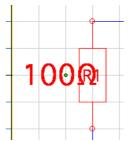
If text is over other object, you can move only it if you maintain the alt key pressed. Edit all the components with the same way. Edit also the 12V, replace with 5V and the label, name it "Output"
